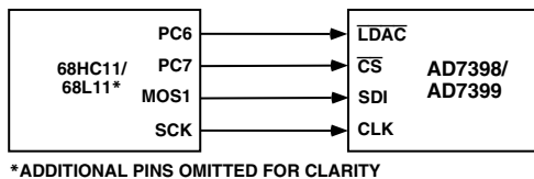
Figure 9. 68HC11/68L11 to AD7398/AD7399 Interface
